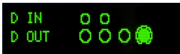
Figure 4-6: Discrete I/O Test Screen, One Output Active
