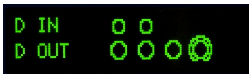
Figure 3-19: Discrete I/O Test Display, Output Active (bottom)
