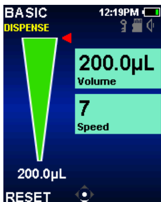
Figure 12: Basic Mode Dispense Operation.
