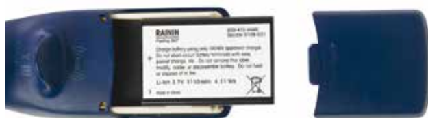
Figure 28: Replacing the Battery
