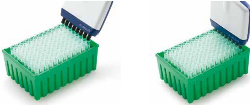
Figure 35: Mounting Racked LTS Tips
